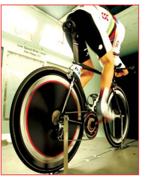
San Diego Low Speed Wind Tunnel Feb 15, 2007. The first true negative drag number ever recorded for a bike wheel.
